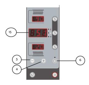
End of cooking time Buzzer The board is equipped with an acoustic signal indicating the end of cooking time (buzzer). To activate it, press and release key (6) when the oven is on. The time (in minutes and tenths of a second) before intervention of the "buzzer" will appear on display (15) and the countdown will automatically activate. If you wish to modify the time, use keys "+" (4) and "-" (5) while display (15) presents the buzzer time. To turn off the oven, hold down key (8) for 2 seconds.
